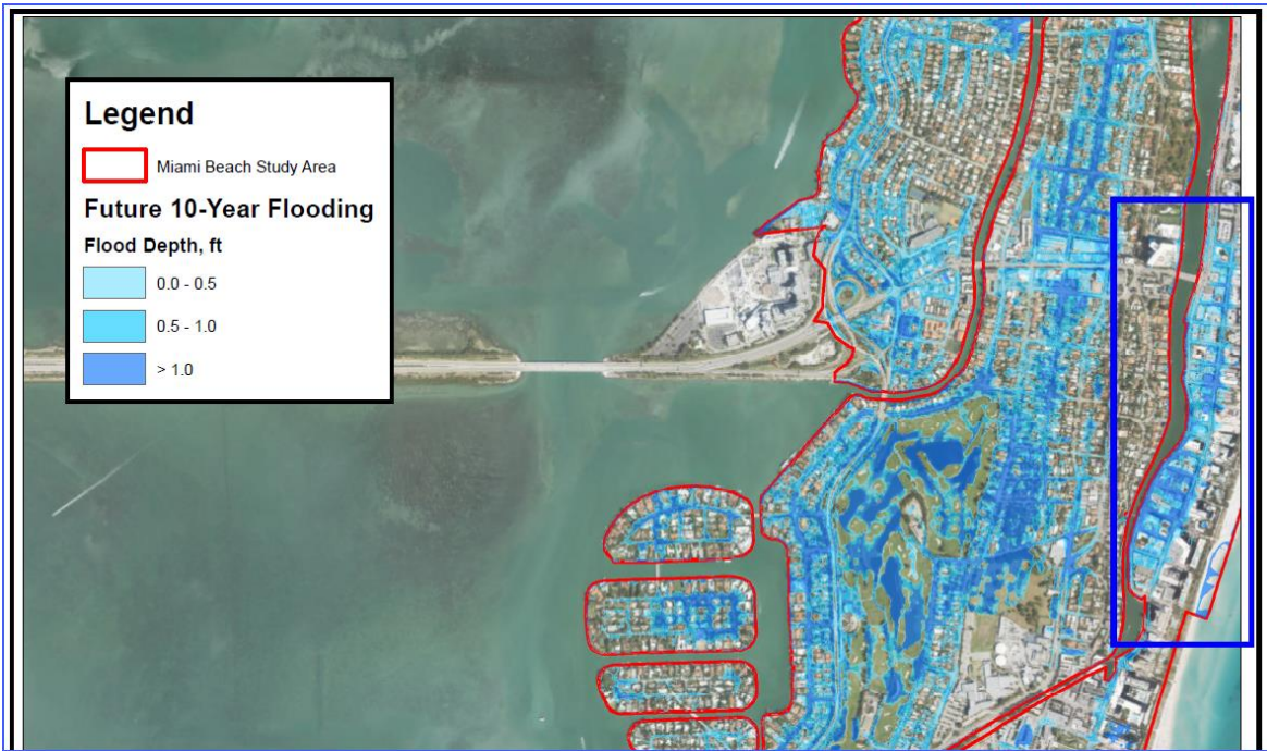
Figure #15. AECOM's Citywide inundation modeling of likely flooding during a 10-year design storm with 8.75 inches of rain in 24 hours.
