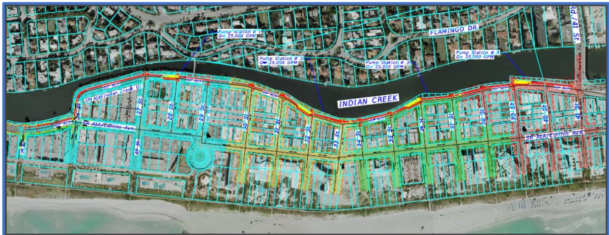
Figure #7. This is a map of a preliminary four-station drainage system proposal that FDOT considered with total pumping capacity of 100,000 GPM, based on a drainage area of 36 acres of public roads and right-of ways. Each station had the capacity to pump 25,000 GPM of water collected from one of four drainage areas, colored in blue, yellow, green and red. It was proposed as a conceptual alternative but later deemed not feasible during the drainage feasibility study.
