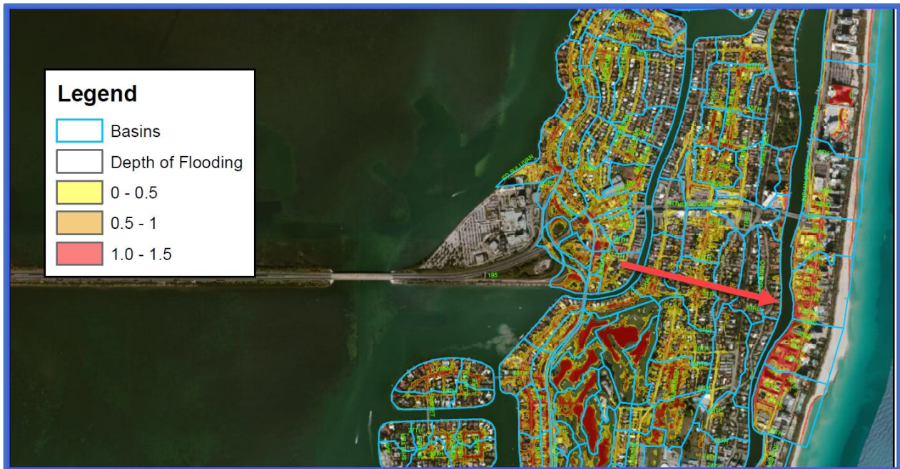
Figure #4. Excerpt from 2015 inundation map titled "AECOM 5-year Simulation – Existing Conditions, North and Middle Beach Locations Not Meeting Level of Service" depicting the expected level of flooding during a storm with the rainfall equivalent to the City's 5-year design storm with 7.5 inches of rain in 24 hours adopted in 2014. The red arrow added here by OIG staff indicates the approximate mid-point of Indian Creek Drive between 25 th St and 41st Street AECOM's modeling showed that areas in red and orange would likely experience flooding of 1 to 1 ½ feet during a 5-year design storm.
