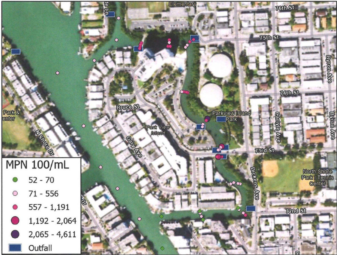
Figure V.2: Map showing measured concentrations of enterococci at the PVC during high tide (August 9, 2022). Hotspots shown by large pink and purple circles.
