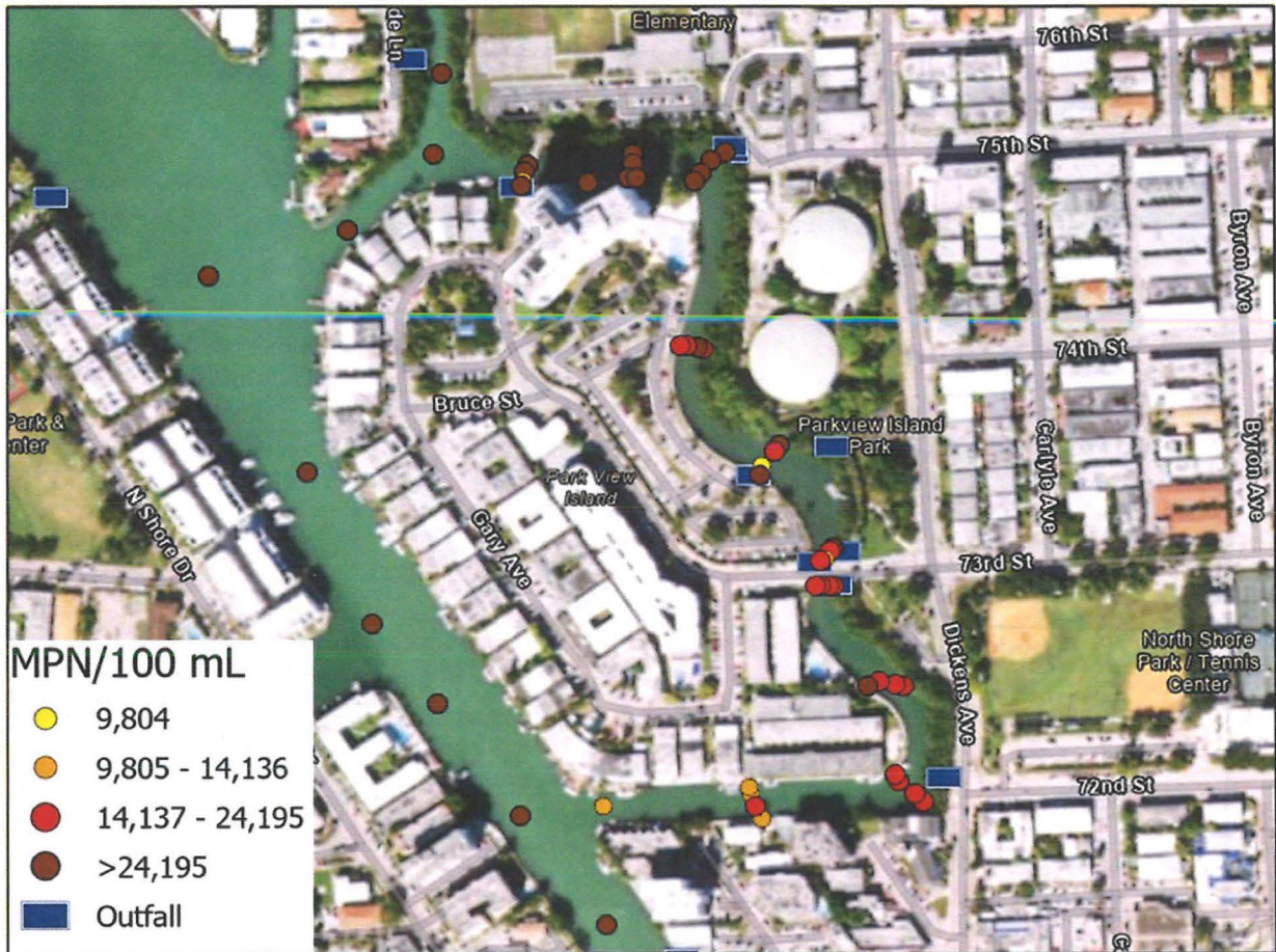
Figure V.3: Map showing measured concentrations of enterococci at the PVC during low tide (September 16, 2022).
